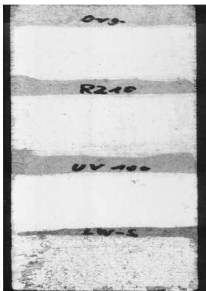
Figure 4. Lime sand stone with four differently pigmented silicate coatings. See text.
